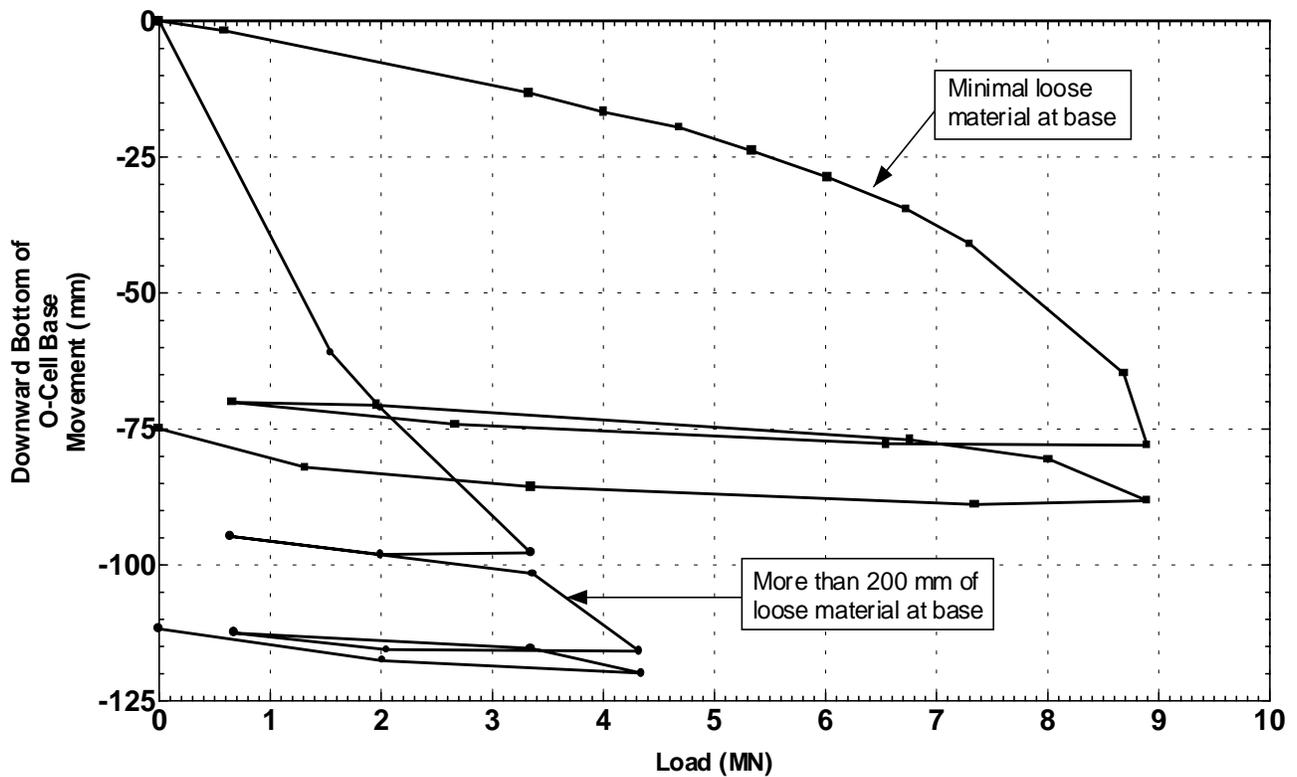
**Fig. 4 - Example 502, effect of poor cleanout ("dry hole") in sands, gravel**
