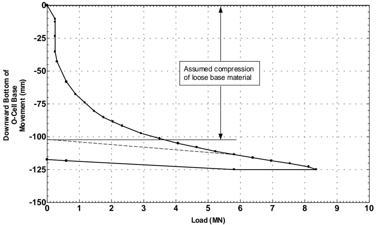
**Fig. 3 - Example 272, effect of poor cleanout procedures ("dry hole") in weathered rock**
